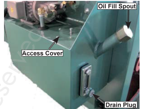
Fig. 71 Headstock oil tank components location
