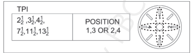
Fig. 61 Opposing number group are selected on dial for cutting 1/2 thread TPI
